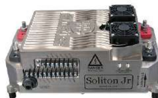
Fig. 8. Electrical Vehicle Controller (3)
