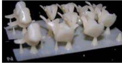
Fig. 24. Applied of Arch models built in plaster like material on 3D Printing system [10]
