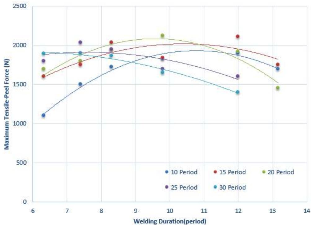
**Figure 3.** Effect of welding time on tensile-peel force
