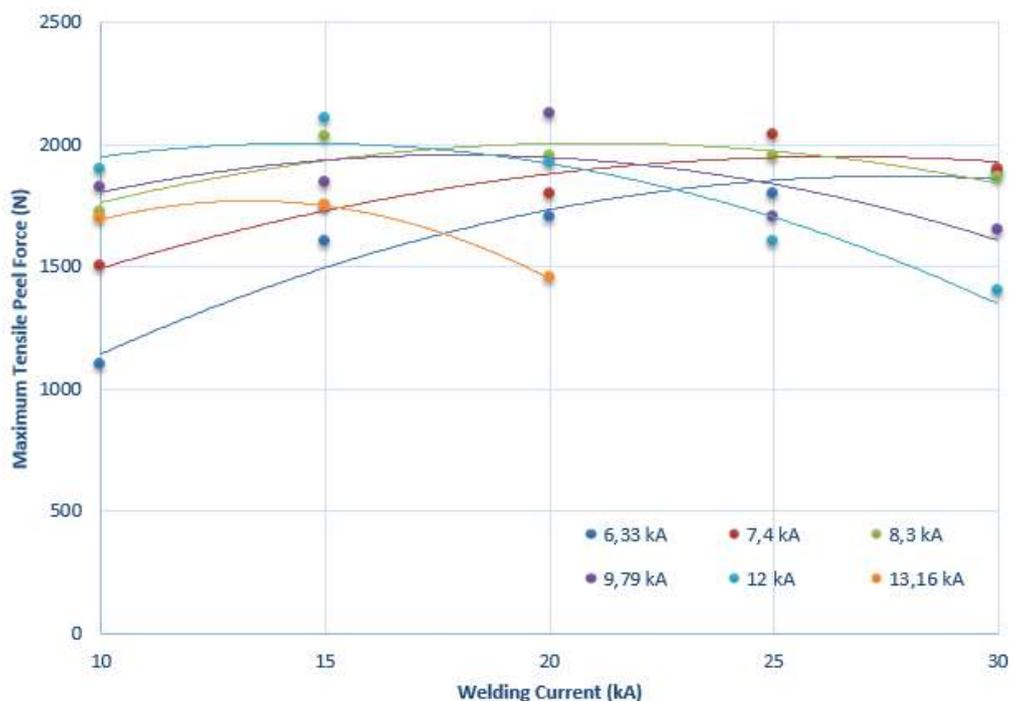
**Figure 4.** Effect of welding current on tensile-peel force
