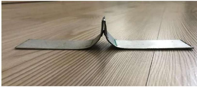
**Figure 1.** Sample of tensile-peel test
