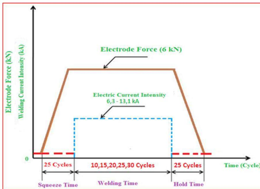
**Figure 2.** Detailed processing parameters
